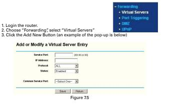
4. Fill in the service port (exception is 80), IP address of camera, then click SAVE. NOTE: The port and IP address should be same as camera.
